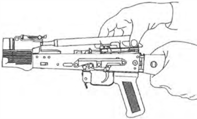
Figure 3.5 – Detaching the bolt support and the bolt
