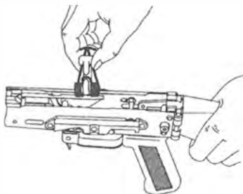
Figure 3.12 – Taking the hammer from the receiver
